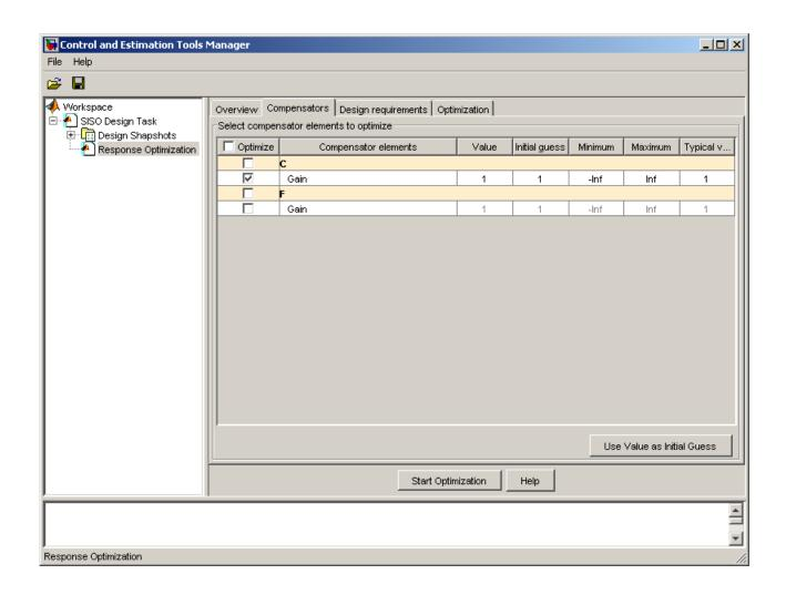
**Note** Compensator elements or parameters cannot have uncertainty when used with frequency-domain based response optimization.
