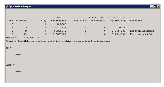
The Optimization Progress window shows the new optimized parameter values of  $0.0034~\text{m}^2$  for the cross-sectional area of the piston, and  $0.0030~\text{m}^3/\text{s}$  for the pump flow rate. These values are also changed within the MATLAB workspace.
