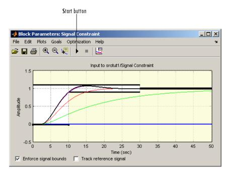
The blue line shows the initial response and the black line shows the current, or final, response. As you can see, the final response signal lies within the constraint bounds.
