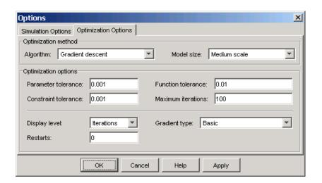
To run the optimization, select **Optimization > Start** or click the **Start** button on the toolbar in the Signal Constraint window. The results, shown below, are similar to the previous ones when only constraint bounds were used.
